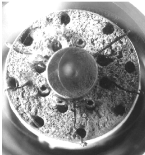
Fig. 9. \text{Al}_2\text{O}_3 porous wick with 8 vapour channels and 8 liquid channels is immersed in a propane pool and heated with an electric heater inside the porous structure. ("inverted" meniscus of evaporation), T_s=303 K, q=1.2 kW/m 2 .
