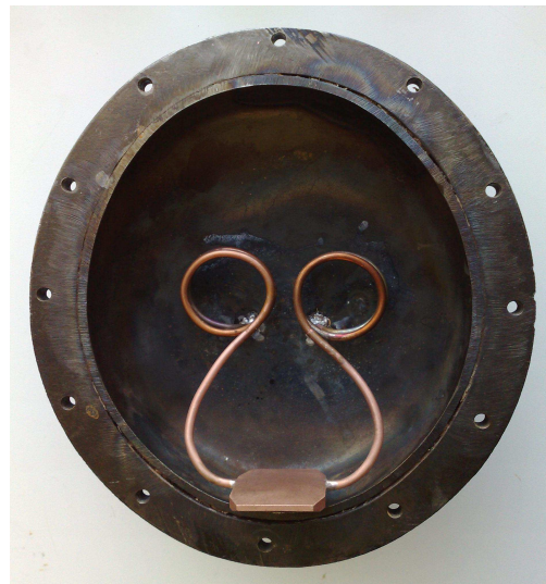
Fig. 6. PLT evaporator and transport zone with two pipes for vapor and liquid transport between the evaporator and condenser
