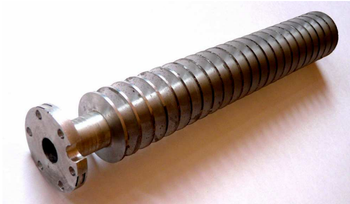
Fig. 2. Transversely finned tube with trapezoid profile fins
