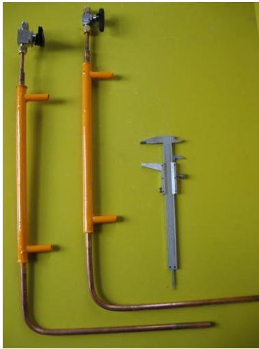
FIGURE 13. VDT with horizontal evaporator and vertical condenser (left) and traditional thermosyphon with horizontal evaporator and vertical condenser (right)
