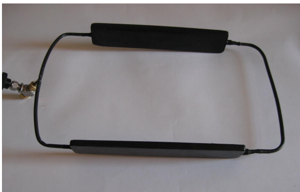
Figure 1a. Flat loop thermosyphon made from polymer composite.
