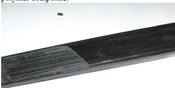
Figure 1a. Flat loop thermosyphon made from polymer composite.
