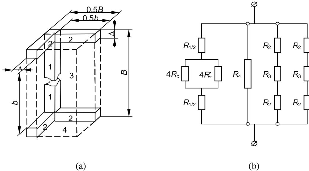
Figure 8. (a) One quarter of the porous coating elementary cell, and (b) diagram of its thermal resistances.
