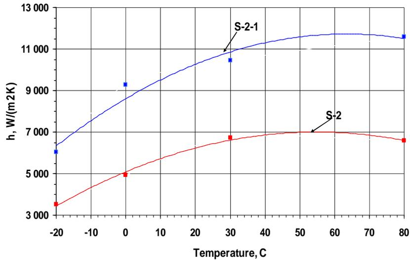
Figure 11. Heat transfer intensity in the evaporators S2 and S2-1 (ammonia) as the function of the saturation vapor temperature
