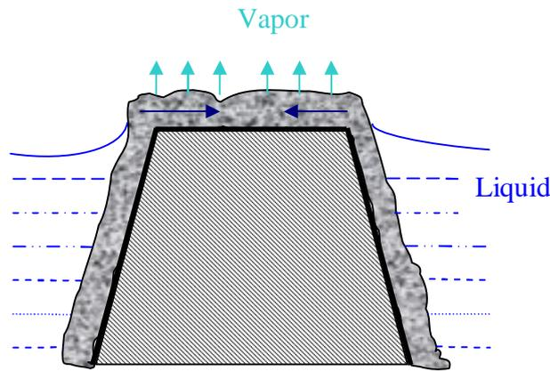
Figure 14: Schematic of the liquid evaporation at the edge of GHP with porous coating
