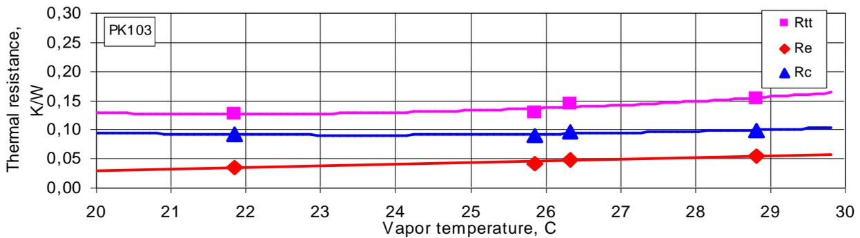
Fig. 20 Thermal resistance of evaporator ( $R_e$ ), condenser ( $R_c$ ) and total thermosyphon ( $R_{tt}$ ) as a function of the vapor temperature in the adiabatic zone (vapor pipe).
