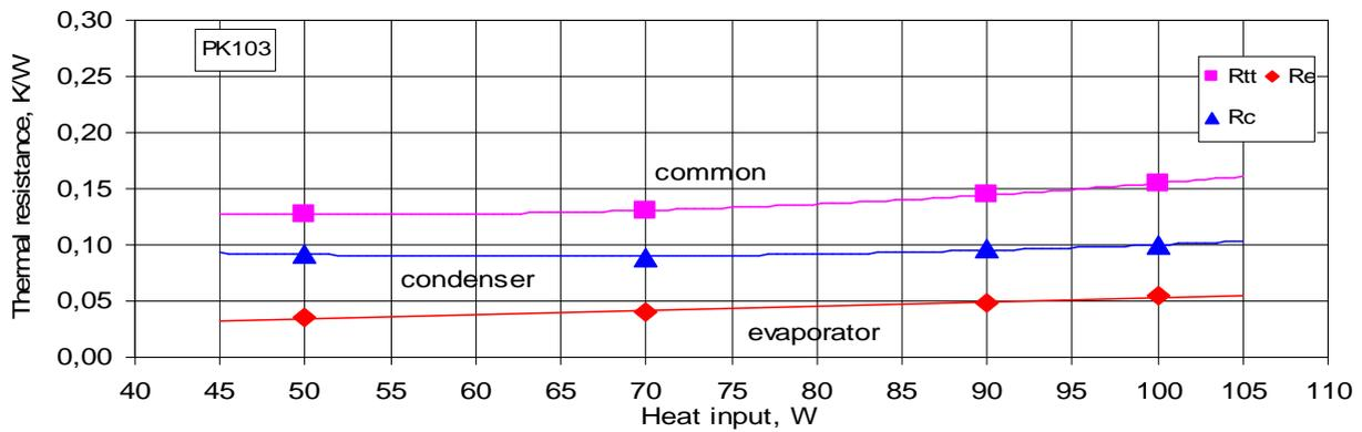
Fig. 19 Thermal resistance of evaporator ( $R_e$ ), condenser ( $R_c$ ) and total thermosyphon ( $R_{tt}$ ) as a function of heat input.
