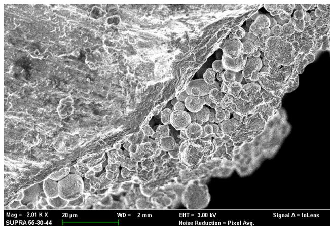
Figure 16. Aluminum oxide porous coating of GHPPL mini groove
