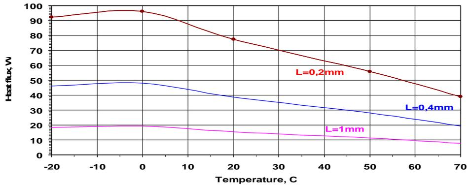
Figure 15. Heat flow removed from one edge of the capillary groove with porous coating as a function of temperature.  $L$  is the edge width, mm; temperature of ammonia vapor  $-20^{\circ}\text{C}$ .
