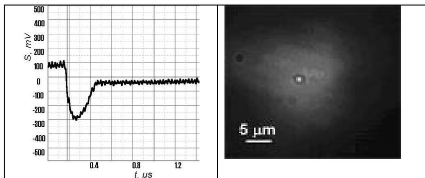
Figure 5. Photo-thermal signals obtained from individual bubble, which was generated in transparent micro-evaporator: PT-response with bubble-specific shape (left) and PT-image (right). Y axis is for the output of the photodetector (mV).
