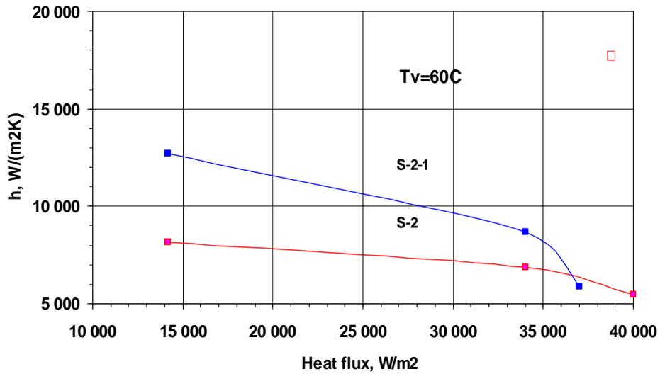
Figure 13. Heat transfer coefficients as a function of heat load in S2 and S2-1.  $T_v = 60\ 0\ C$ .
