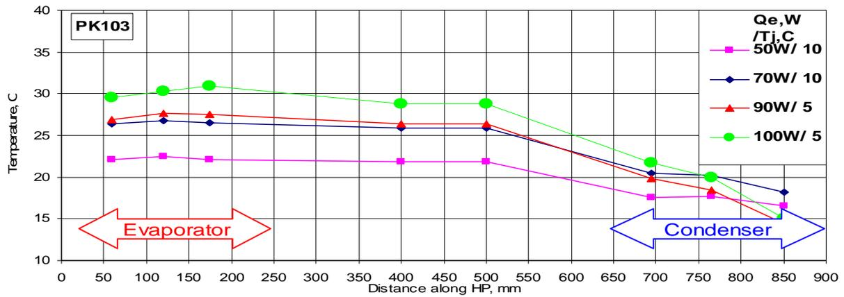
Figure 18. Temperature distribution along the evaporator, transport zone and condenser of the thermosyphon as the function of heat input.
