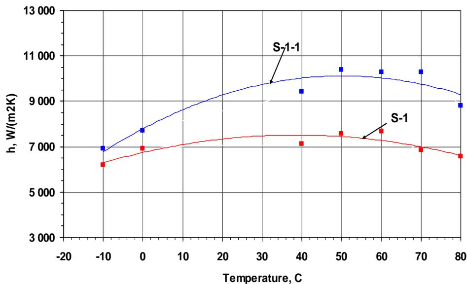
Figure 10. Heat transfer intensity in the evaporators S1 and S1-1 (ammonia) as a function of the temperature of saturated vapor
