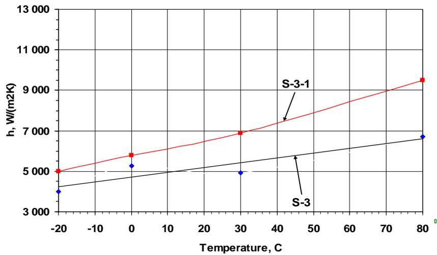
Figure 12. Heat transfer intensity in the evaporators S3 and S3-1 (ammonia) as function of the saturation vapor temperature
