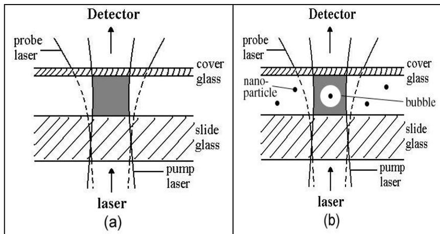
Figure 3. Visualization of the bubble generation by short laser pulse (532 nm, 10 ns) in mini channel of the flat evaporator with nano fluid (water +  $\text{Al}_2\text{O}_3$  NPs) .(a) - control pure water; (b) – nano fluid;  $D_{\text{Al}_2\text{O}_3}$  particle < 220 nm.
