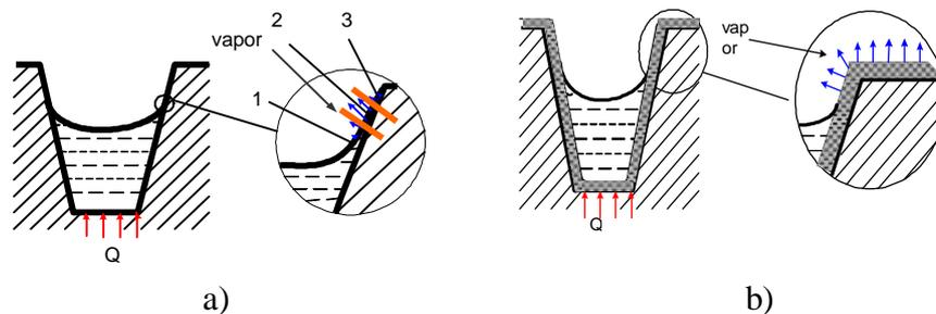
Figure 6. Evaporation phenomena in trapezoidal grooves: (a) smooth; (b) with porous layer. 1- liquid meniscus, 2 - thin film – zone of extensive heat transfer with evaporation, 3 –dry zone of groove
