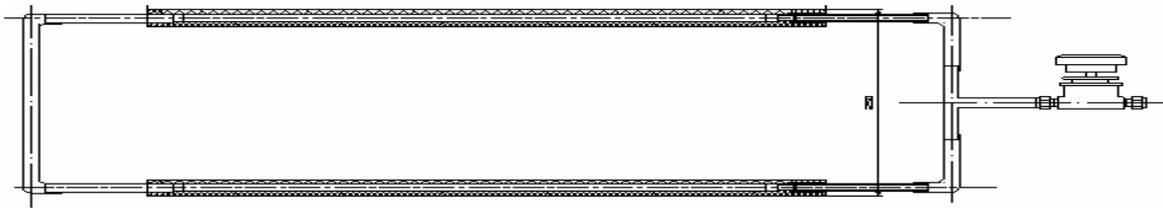
Figure 17. Flat loop thermosyphon made from polymer composite
