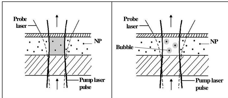
Figure 4. Experimental model: laser-induced heating of the volume of liquids with non-absorbing nano particles  $\text{Al}_2\text{O}_3$  (left); generation of laser-induced bubbles around gold light-absorbing nano particles (right); single laser pulse: 532 nm, 10 ns.
