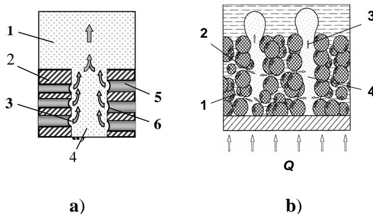
Figure 7: Model of heat transfer on the edge (a) and bottom (b) of the GHP mini groove with porous coating.
